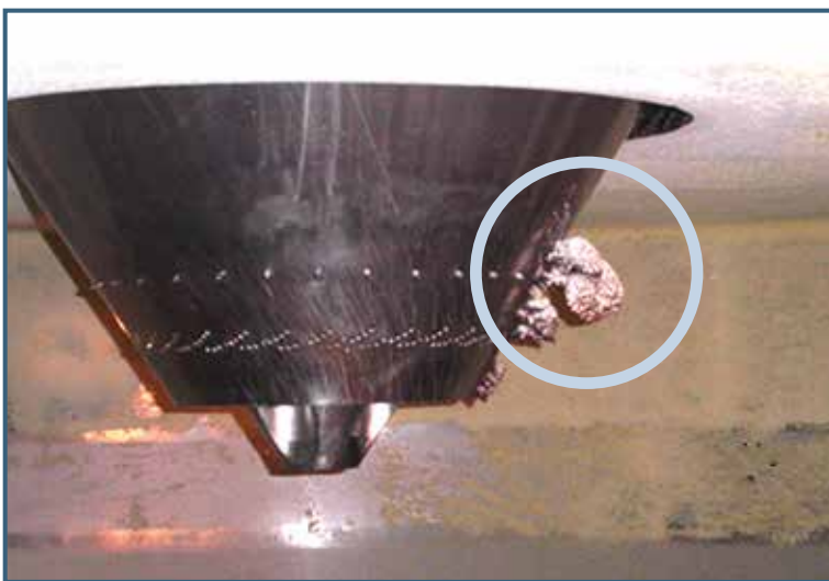
Smoldering deposit detected by ACOM Early Fire Detection System
